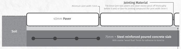
5 - 10mm **Premium Cement Based Tile Adhesive** -Applied with 10mm+ notched trowel or 10-20mm bed of mortar - must be thick enough to allow adjustment for +/-2mm variation in thickness of pavers
