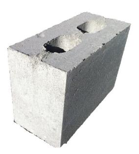
📕 110mm **Bare Wall** 45 Rw 2 x 13mm Boral Plasterboard 46 Rw daub fixed Boral Impact Clip with 28mm furring channel 49 Rw one side, daub fixed on other side. Boral Impact Clip with 28mm furring channel and TSB3 51 Rw polyester insulation one side, daub fixed on other side. Boral Impact Clip with 28mm furring 52 Rw channel both sides. Boral Impact Clip with 28mm furring channel and TSB3 57 Rw polyester insulation both sides. 48 Rw\* 2 x 13mm render both sides.
