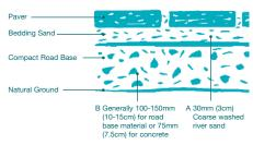
Tip: It is essential that rain water flows off the paving and away from buildings. To ensure this paving must not be completely flat, it should slope away from building. If the paving is against the side of a building, the pavers need to be a minimum of 25mm (2.5cm) below the damp proof course to prevent rising damp problems in your home. The damp proof course and air vents should never be covered.
