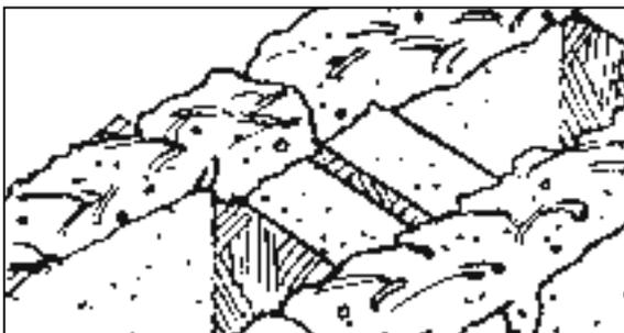
Figure 3 Mortar applied to the face-shells
